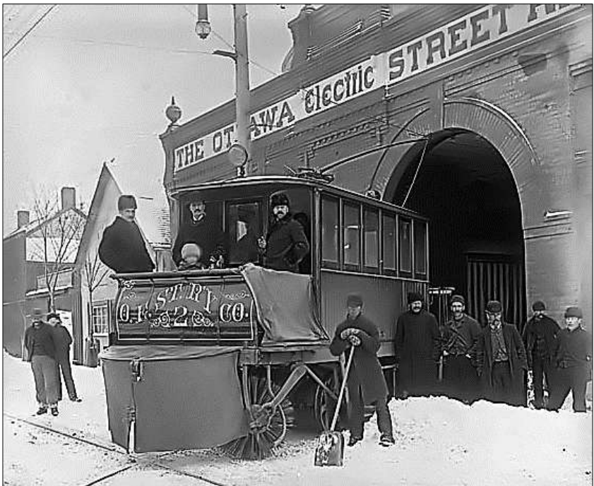
Ottawa Electric Railway Streetcar with rotary snow sweeper, c 1895 (Library and Archives Canada, PA-173828)
